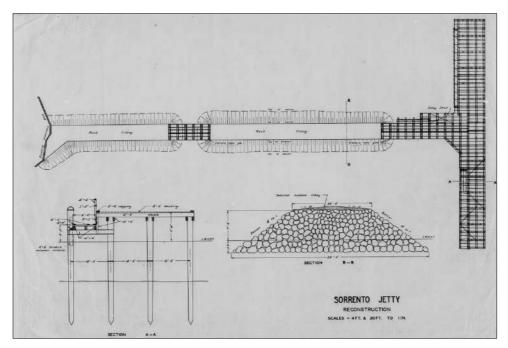
Figure 19 A 1952 drawing for the replacement of most of the pier with a rock mole. Source: Parks Victoria.
