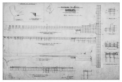
Figure 10 A 1904 plan for repairs to the Sorrento Pier, also appearing to involve pile replacement as well as new planking. Source: Parks Victoria.
