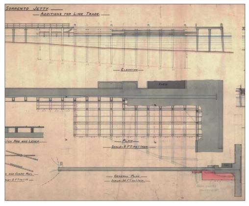
Figure 7 1886 drawings for enlargement of the deck to Sorrento Pier for the lime trade. Source: Nepean Historical Society
