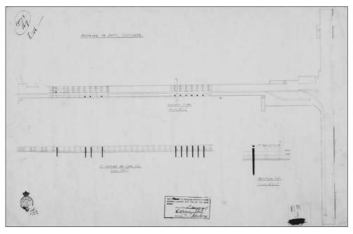
Figure 14 A 1907 drawing for repairs to the pier, presumably limited to replacement of piles. Source: Parks Victoria.
