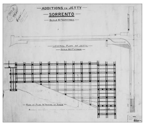
Figure 16A 1912 drawing showing extensions to the deck (at the junction of the T-head) and to<br/>the end of the east arm.<br/>Source: Parks Victoria.
