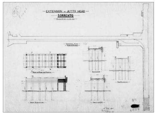
Figure 15 A 1910 drawing showing an extension to the east arm of the T-head. Source: Parks Victoria.
